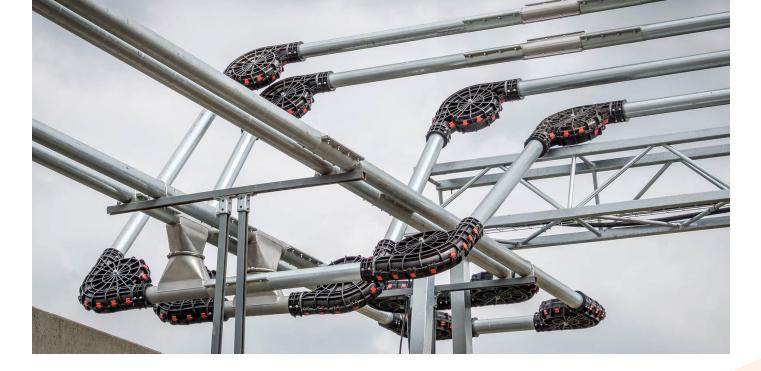
Tubular conveyor consists of a series of circular discs, equally spaced between them and attached to the chain, which gently drag the product along the path.
